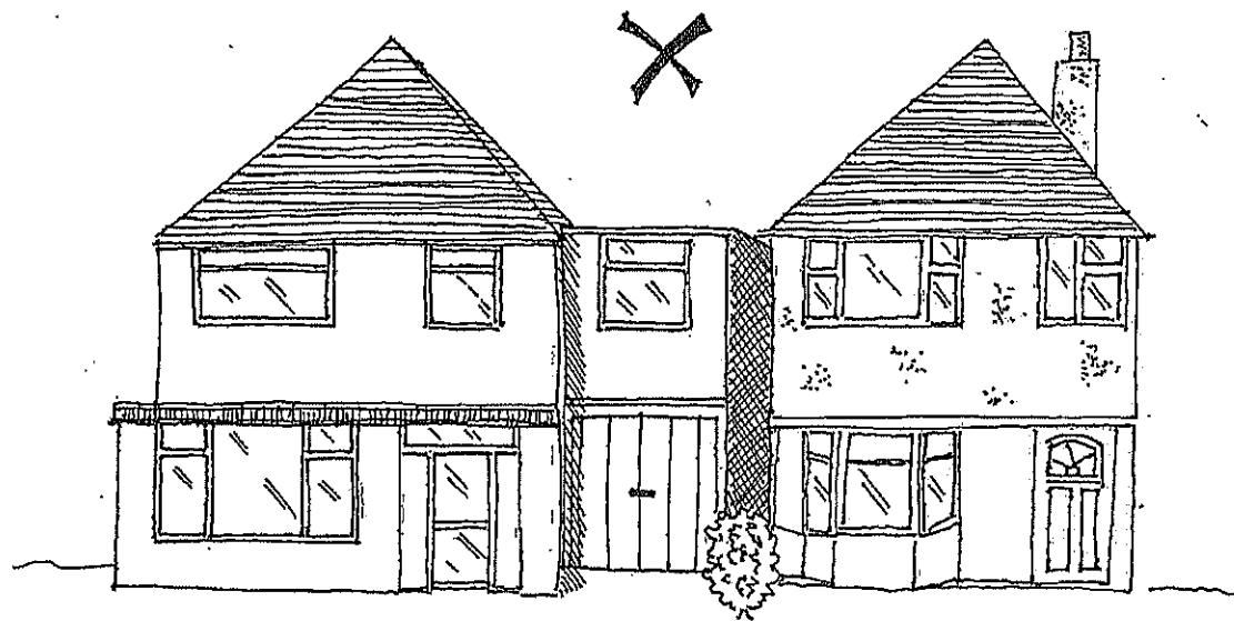
Fig. 5 -Unacceptable flat roof extension
